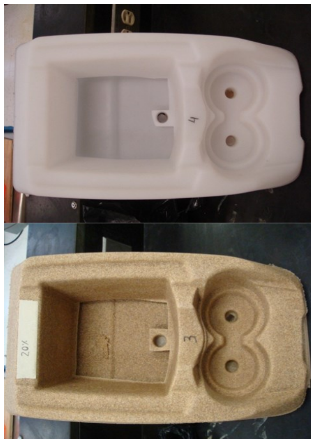
Figure 2. Typical parts produced by rotational molding with 0% wood (left) and 20% wood (right).
