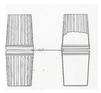
There are, however, large quantities of opentopped tanks, drums, containers and other products produced by rotational molding. It is a common practice to mold a long, cylindrical or square part that is cut in the center to produce two shorter containers open at one end. The two refuse containers shown in Figure 1 were produced using this technique. It is even more common to mold a tank of the required size and then cut a large opening in one end (Figure 2A).
